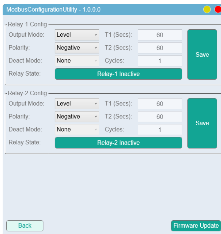
Figure 19 - Modbus 2CH Relay Control Window
