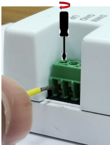
Figure 8 - Clamping wire with screwdriver in clockwise direction
