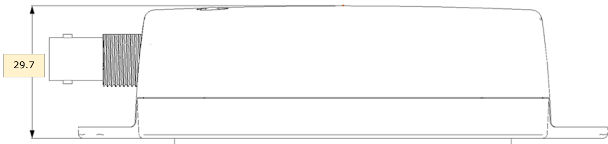
Figure 7 - Modbus Salinity Sensor Adapter Dimension – Side View
