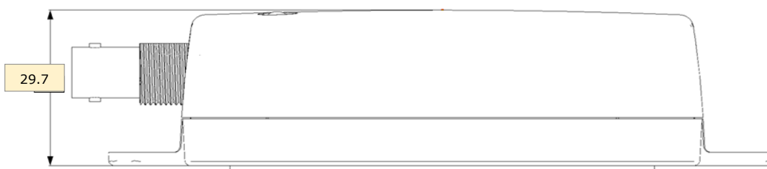
Figure 7 - Modbus pH Sensor Adapter Dimension – Side View
