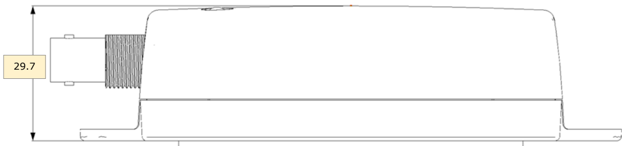
Figure 7 - Modbus EC Sensor Adapter Dimension – Side View
