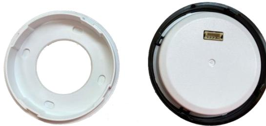
7. Connect the JST cable from the top section of the swivel mount to the JST connector located on the back of the device.
