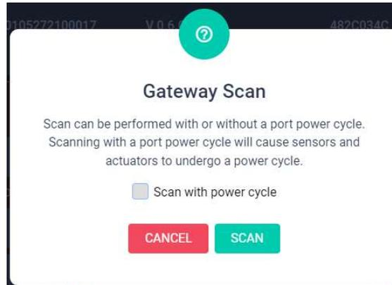
Scan without Power Cycle: De-selecting this checkbox will just discover all the connected devices on all the 3 ports.
