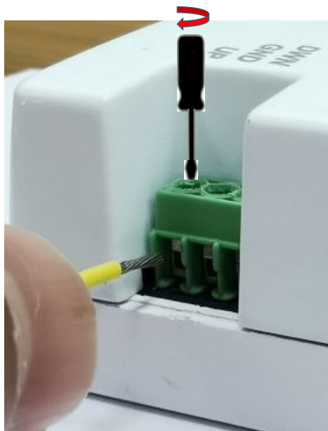
Figure 7 - Clamping wire with screwdriver in clockwise direction
