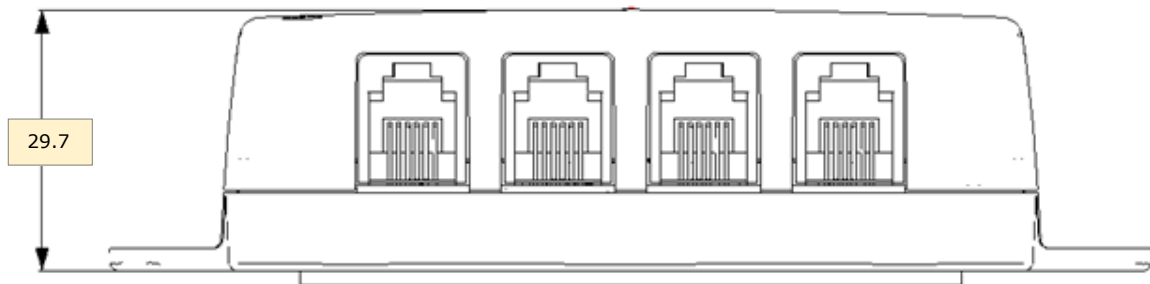
Figure 6 - LDSBus Quad T-Junction 2 Dimension – Side View
