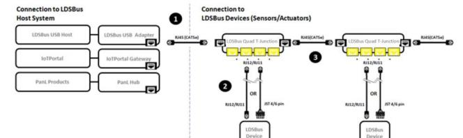
Note: Enable termination for last LDSBus Device in the bus
