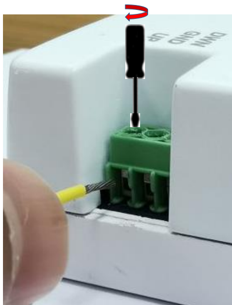
Figure 7 - Clamping wire with screwdriver in clockwise direction
